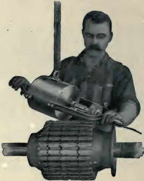
FIG. 343.—Portable Grinder (Cleveland Armature Works).
